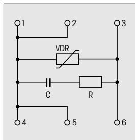
RC-element parallel to voltage absorber (Varistor)
