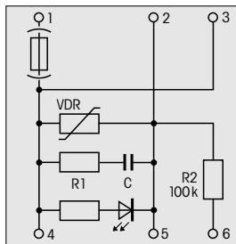
Combination with fuse, LED and shunt resistor
